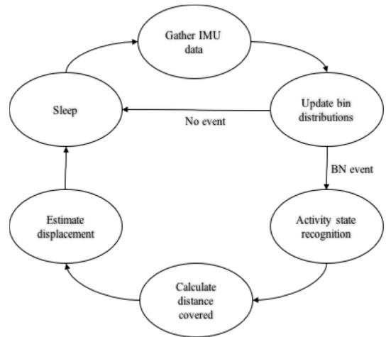
Fig. 2. State diagram for on-board analysis on wearable devices
